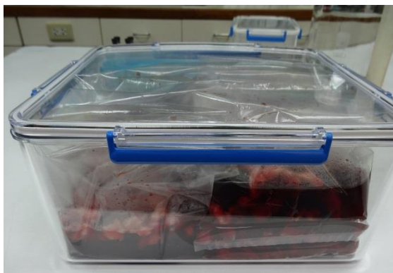
Figure 3. Enriched with Bolton broth and incubated at 42°C for 48 h
