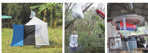
Fig. 2 NZI trap (left), CDC (middle) & modified light (right) traps
